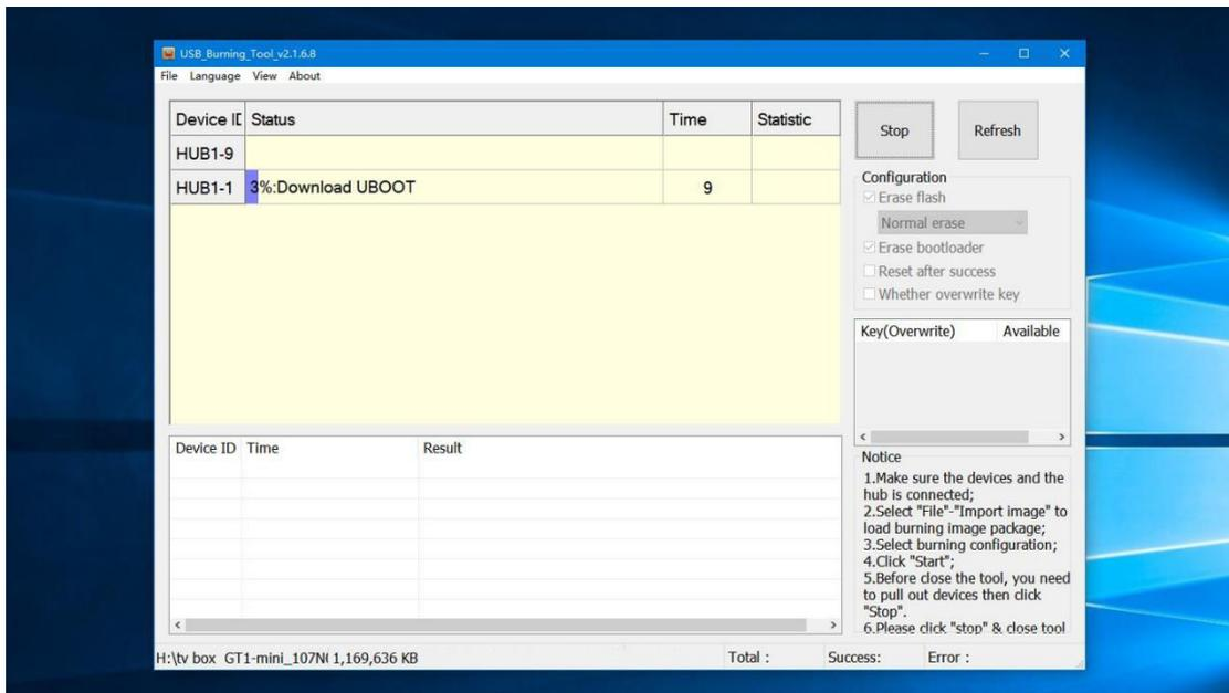
10.Load 100%, unplug the GT-King USB cable and power cable, click stop, close the tool, and finish the brush.
