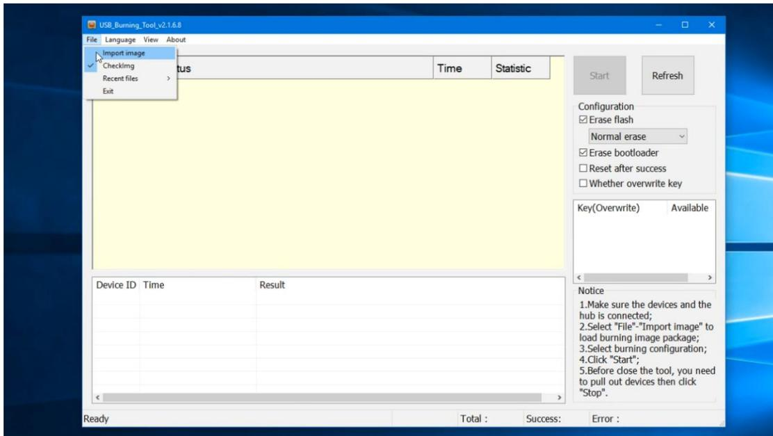
6. Load the firmware, click Import image to enter, find the downloaded USB cable brush firmware location, select and click to open, as shown below
